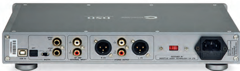
ABOVE: USB and both Toslink and coaxial S/PDIF digital inputs are joined by a coaxial digital output, single-ended analogue line in, line out and balanced line out on XLRs
